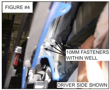
STEP #4: Pull the wheel well cover back. Locate and remove the (3) 10mm fasteners securing the fascia to the fender. See Figure #4. Repeat for passenger side.
