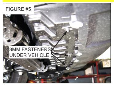
STEP #5: Move to the under carriage of the vehicle. Remove the plastic skid plate. Locate and remove the (3) 8mm fasteners shown in figure #5. Pull firmly on the outer edge of the fascia and remove from the vehicle.
